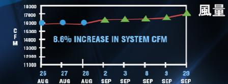
Measurements taken for 3 days 8/26-8/28 to establish the baseline. The UVC Emitters™ were installed in the afternoon of 8/29.
